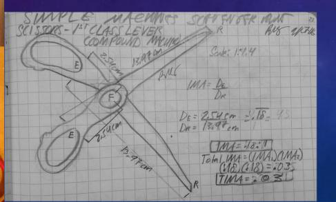
Since this is a compound machine, you must multiply both IMAs to get the total IMA. Since each lever has the same effort distance and resistance distance, that would be (.18)(.18) or .03 so the total IMA of the scissors is .03
